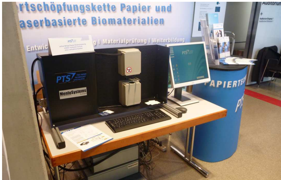
Figure 2: Encapsulated measurement setup of the PTS for online applications and for 2D and 3D imaging, using Menlo Systems' TERA K15 THz-TDS-System.
