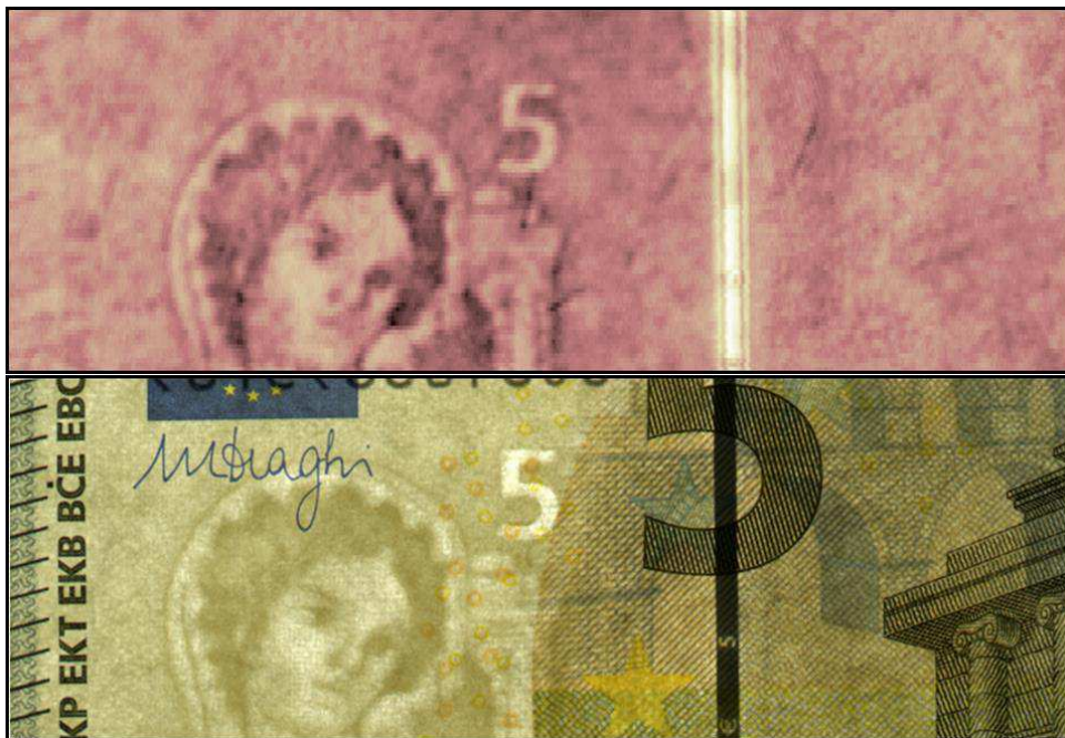
Figure 4: THz transmission image and backlight image of a watermark on a 5 Euro bank note, sample size: 70 \text{ mm} \times 24 \text{ mm} .
